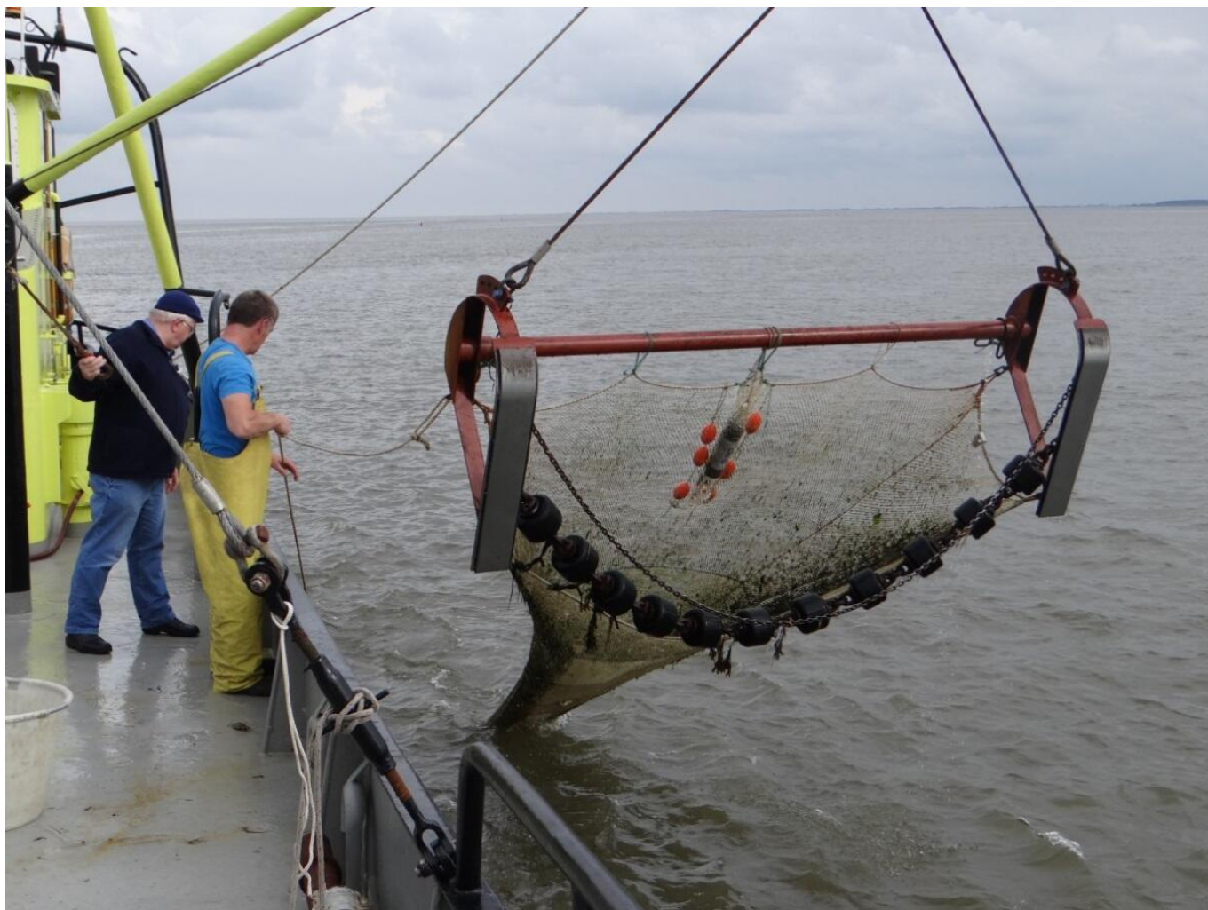
Figure 5. The 3 m beam trawl deployed in the Dutch Demersal Fish Survey (Photo: Ingrid Tulp, IMARES).
