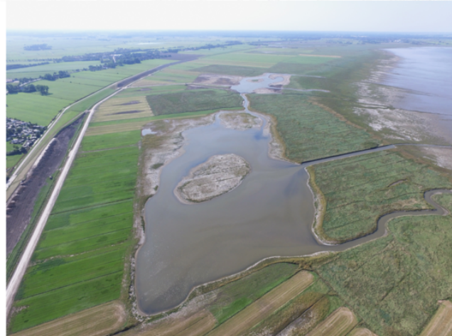
Figure 15. Example of re-designing and rewetting an artificial salt marsh after clay extraction by removing the top soil in the Neuwapeler Außengroden, Jadebusen, Lower Saxony. The photo shows the re-designed sections A and B (90° rotated). (Photo and schematic overview: Planungsgruppe Grün, Herr Sprötge; legend translated and modified by the authors).
