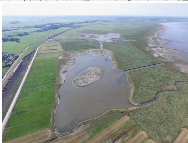
Figure 15. Example of re-designing and rewetting an artificial salt marsh after clay extraction by removing the top soil in the Neuwapeler Außengroden, Jadebusen, Lower Saxony. The photo shows the re-designed sections A and B (90° rotated). (Photo and schematic overview: Planungsgruppe Grün, Herr Sprötge; legend translated and modified by the
