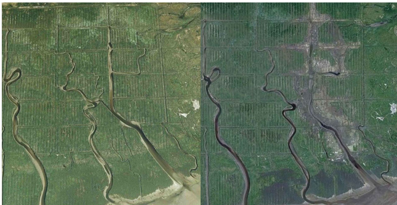
Figure 10. Restoration of natural drainage in the back-barrier salt marsh on island of Norderney, Lower Saxony. The top soil was removed to decrease the artificial drainage (Linders et al. , 2013). Left: situation in 2008 before restoration (Photo: 2017 GeoBasis-DE/BKG on Google Earth), right: situation in 2015 after restoration (Photo: 2017 Earthstar Geographics SIO on Bing Maps by Microsoft)
